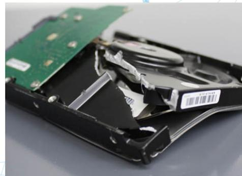
HDDs that have been both degaussed and crushed are unrecoverable
